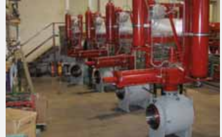
12" 150 Fully Welded Body
