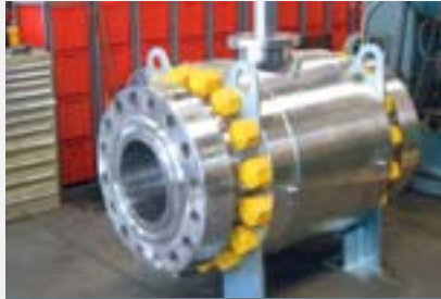
16" 1500 Fully Duplex Metal Seated
