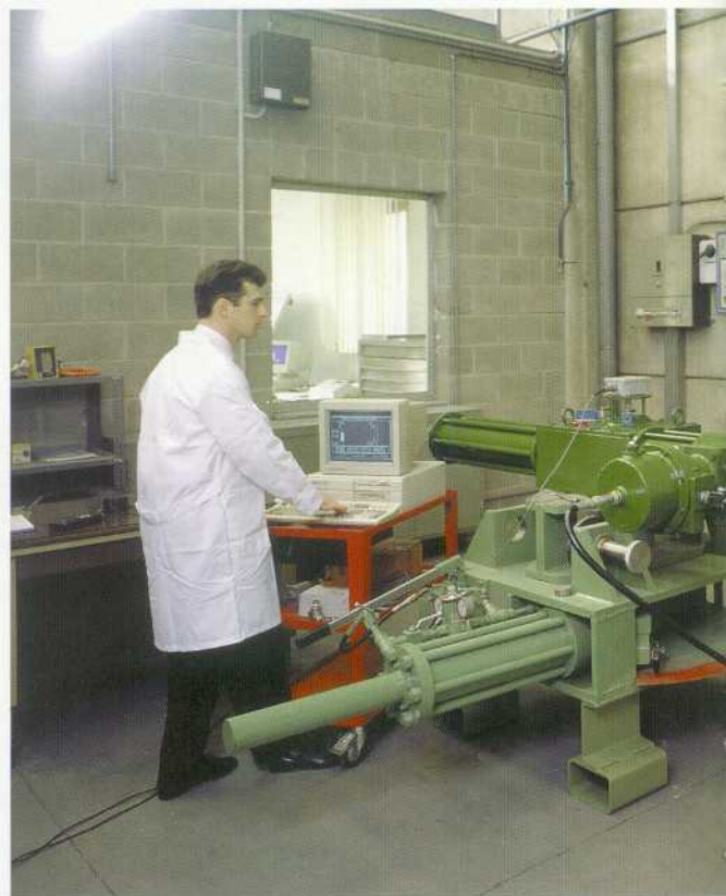
RHMS actuator during torque test (emergency stroke time 0,2 sec)
