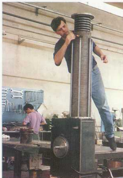
Assembling of RHM 3000/180 cup spring cartridge
