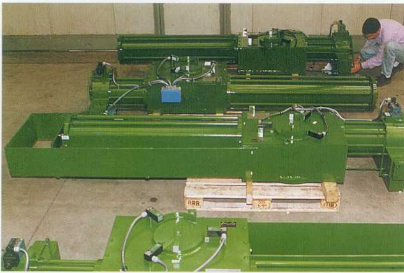
Modulating RHMS 5000/250 with quick emergency closure (stroke time 0,2 sec)
