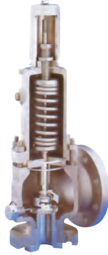
Starflow P3 / P4 / P5 ASME Section VIII Div. 1 (UV Stamp) API Std 526 Full Nozzle Inlet size : 1" to 12" Rating : 150# to 2500# Temp : -196°C up to +540°C
