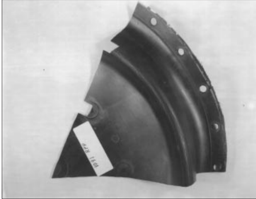
Figure 7-25 Photograph of Crazed Surface of a Section of an OV Diaphragm Removed from Service during ISI
