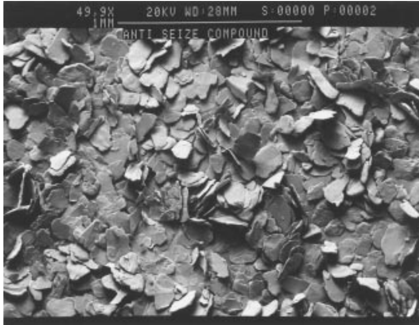
Figure 7-28 View of Graphite-Type Lubricant Film on the Surface of an AOV Diaphragm after Drying
