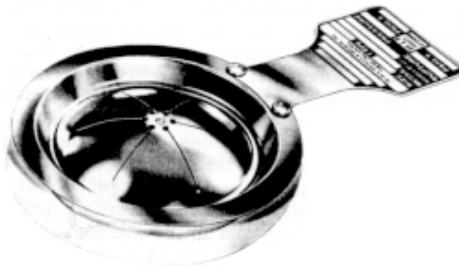
Fig. 10-8. A composite rupture disc has a weakened metal disc backed by another metal or plastic disc that performs the sealing function.
