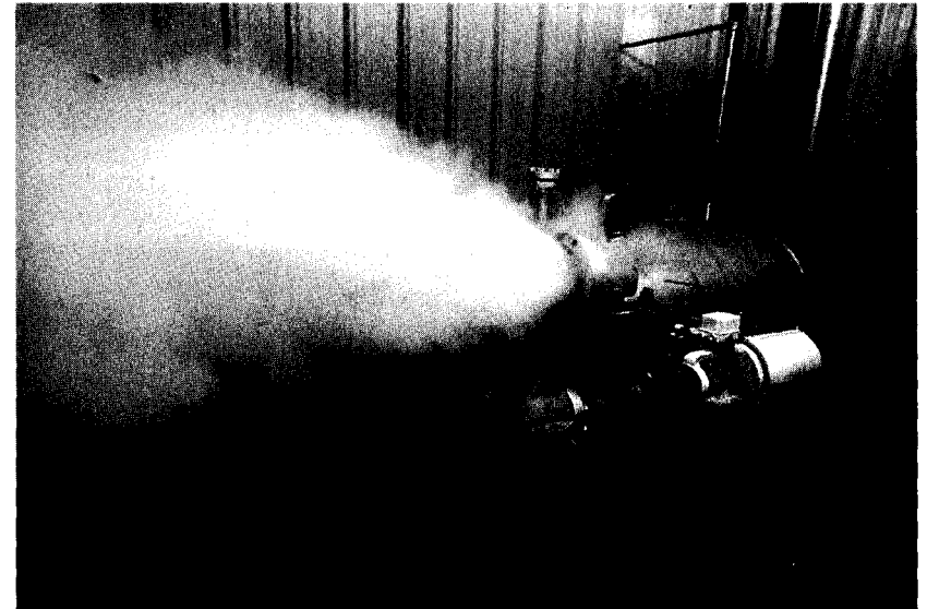
Figure 1.7 Pressure-relief valve being tested for correct cracking pressure. (Courtesy of Valtek Houston Service Center)
