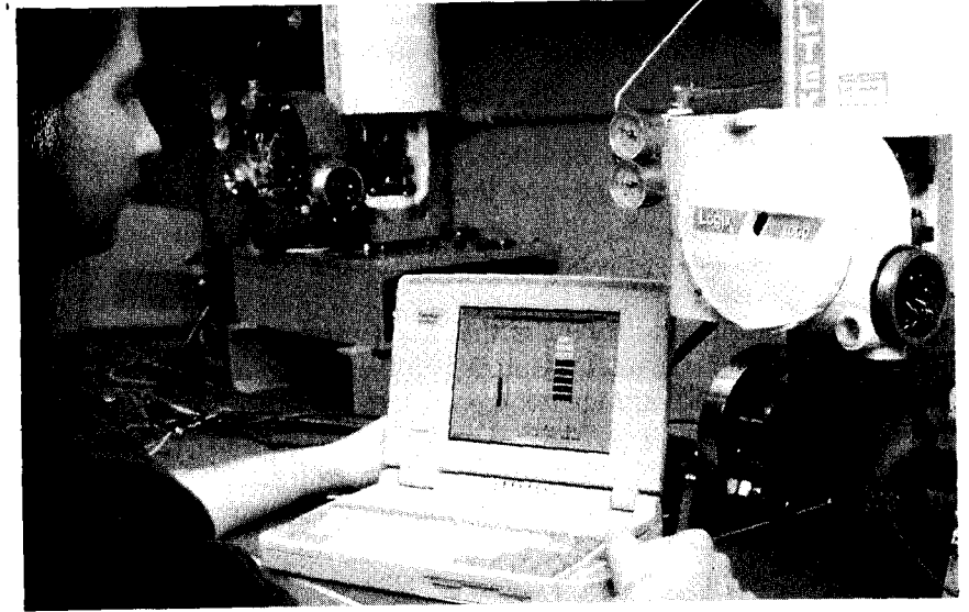
Figure 8.7. Computer interface with a digital positioner. (Courtesy of Valtek International)
