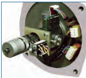
Contactless Position Sensor and Auxiliary Switches
